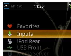
**Coax 1, Coax 2** and **Optical** are all digital inputs for stereo (2-channel) digital sources such as CD, Minidisk, DAT or TV set top boxes. Please note that any connected TV or home theatre related equipment including set top boxes *must* be set up to output a 44.1kHz *or* 48kHz **PCM STEREO** digital stream or similar. The M1 CLiC *does not* recognize multi channel digital audio.
