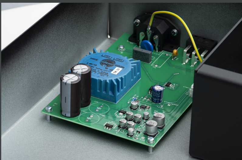
Special Phono Stage PSU Design with Low Core Saturation Toroidal Transformer to Minimize Electromagnetic Radiation
